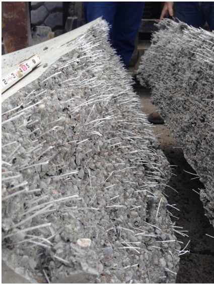
Macro synthetic fibre reinforcement in concrete.
